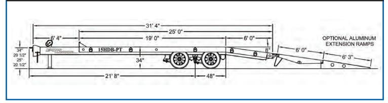
Capacity: 30,000 lbs. Trailer Weight: 8,100 lbs. Deck Width: 8 ft. 6 in. Length: 19 ft. Height: 34 in.
