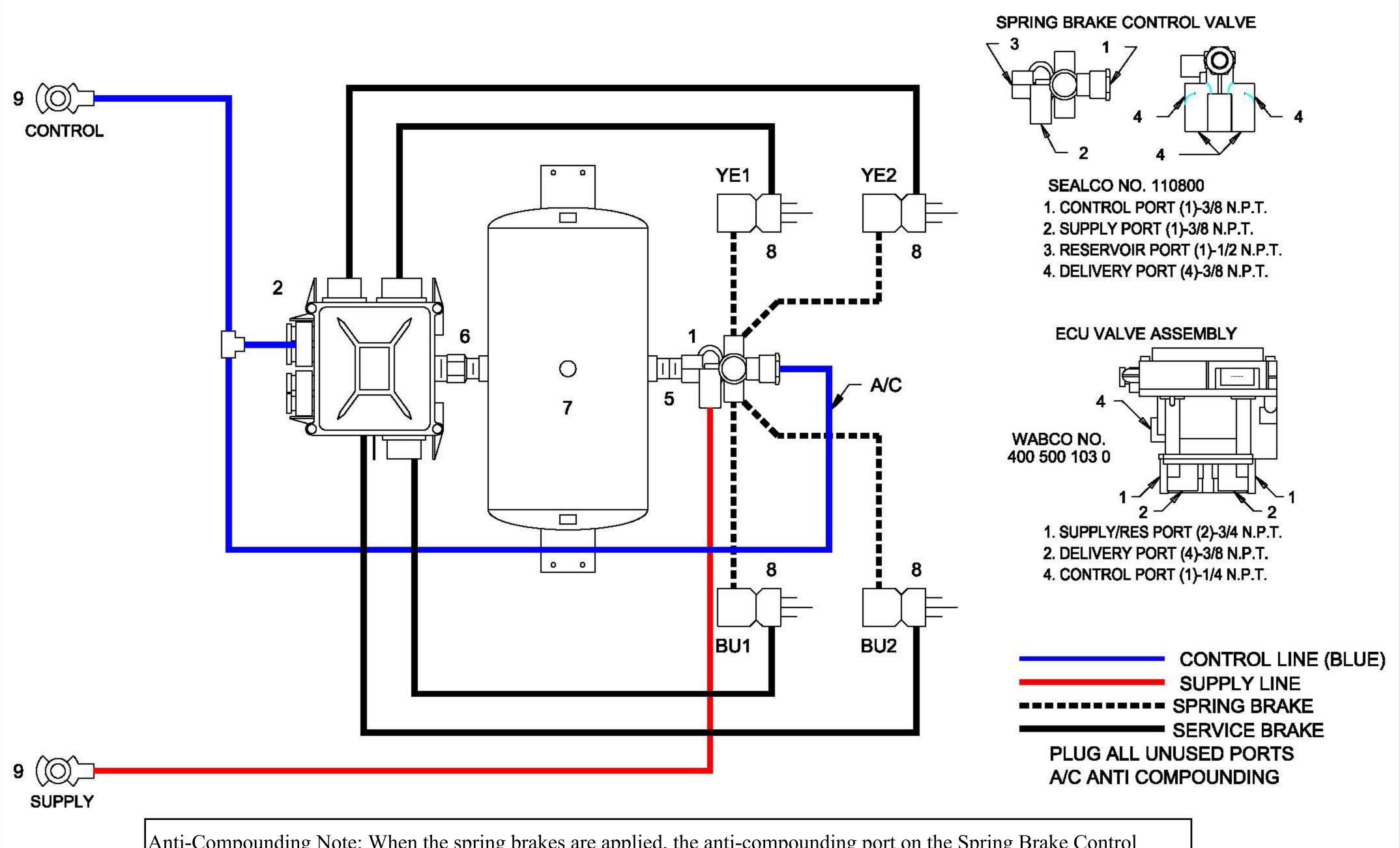
Anti-Compounding Note: When the spring brakes are applied, the anti-compounding port on the Spring Brake Control Valve disables the blue control line air by venting it to atmosphere. This prevents the compounding effect of applying service brakes when when the spring brakes are enabled. Control air will be heard during this venting.
