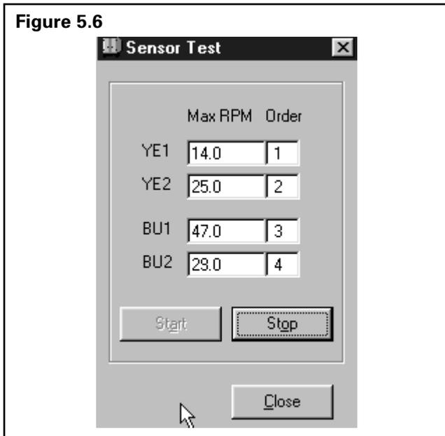
The Sensor Test screen is used to determine the correct installation, wiring and functionality of the wheel speed sensors.
