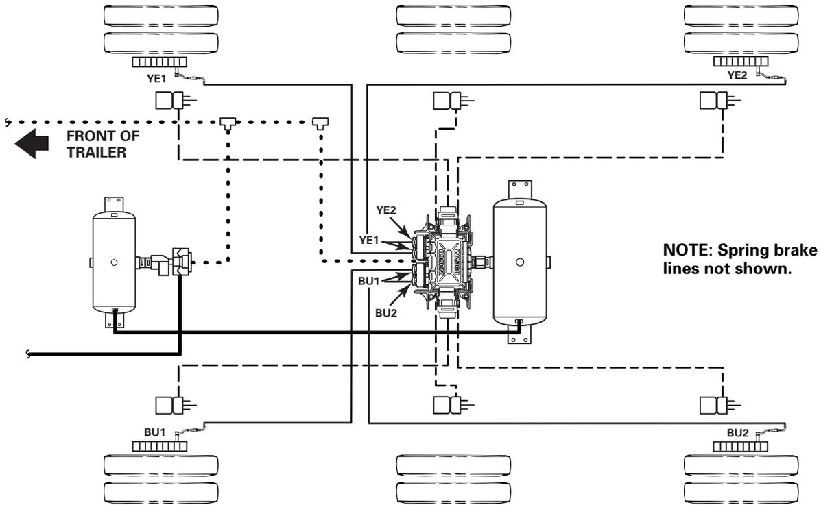
**4S/2M PREMIUM — TYPICAL TRI-AXLE — MOUNTED WITH SENSORS FACING REAR OF TRAILER**
