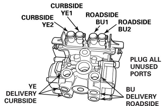
**Figure 7.11****ECU/DUAL MODULATOR VALVE MOUNTED WITH SENSORS FACING REAR OF TRAILER**
