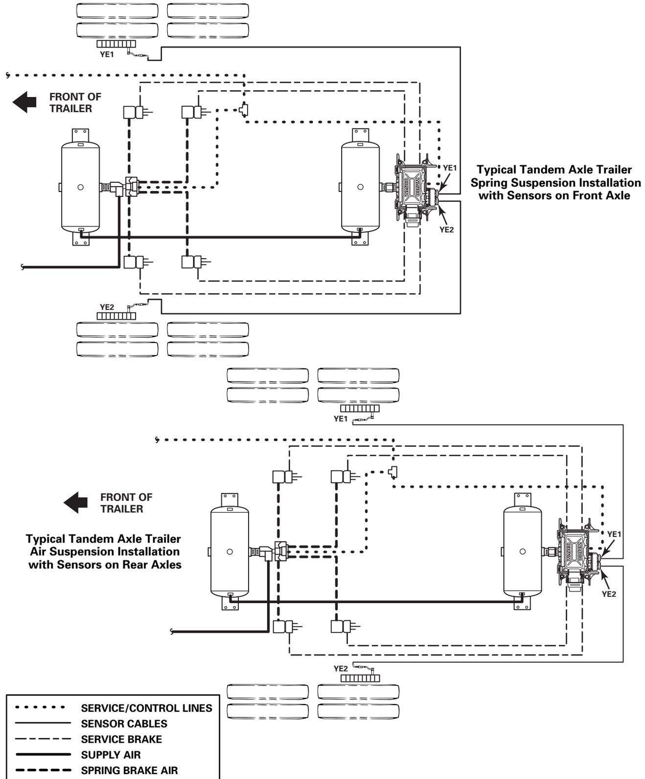
**NOTE:** Meritor WABCO recommends placing sensors on the axle that will provide the most braking performance. The suspension manufacturer can provide this information.
