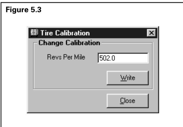
The programmed number of tire Revs Per Mile is displayed on the Tire Calibration screen. Range is 150.0 to 634.0 rpm. The default value is 502.0. To change this value, type in the Revs Per Mile, then press the Write button. **Figure 5.3.**
