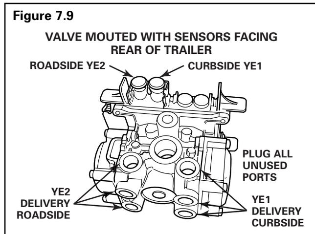
**Inspect the Sensor and Air Line Installation (2S/2M, 4S/2M and 4S/3M Premium)****Sensor Installation**
