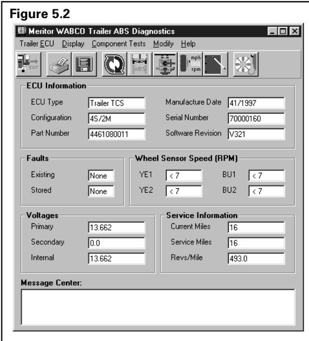
This screen provides icon and pull-down menu task selections. It also provides information about the current state of the Meritor WABCO Enhanced Easy-Stop Trailer ABS. ECU information is read once from the ECU and does not change. Wheel speed, voltages, faults and information are read and updated continuously.
