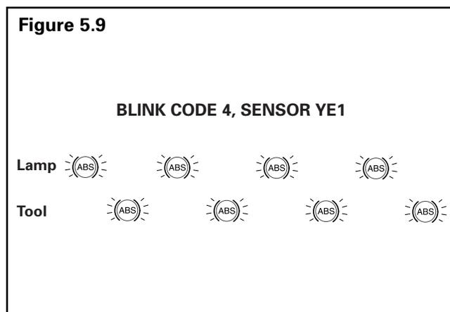
Although the ECU can store multiple faults in its memory, it only displays one blink code at a time. This is why it is important to recheck the blink codes after repairing a fault. If there are additional codes in the memory, they only blink after you have repaired the first fault.
