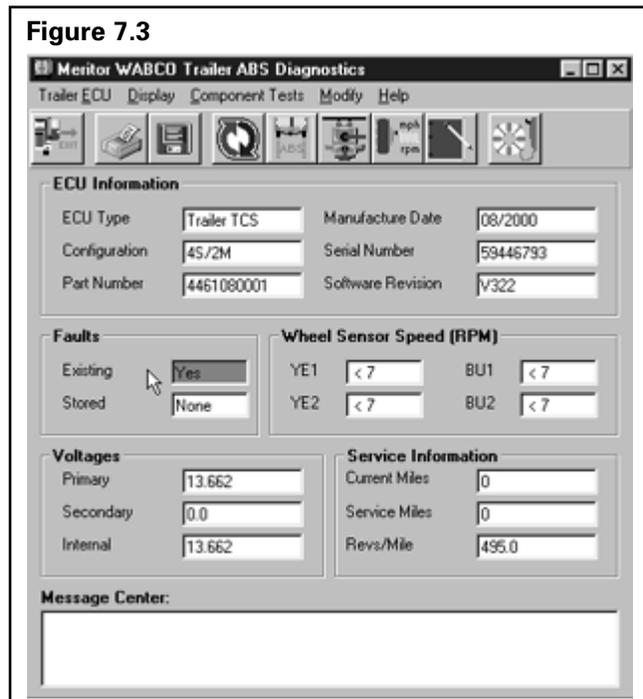
Use the information in the **Repair Instructions** field to make the necessary repairs. **Figure 7.4.**
